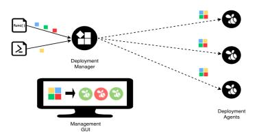
The manager is a centralized web service exposing APIs and a GUI for various deployment-related operations, ranging from compilation to installation and runtime. Deployment agents run on individual devices, performing deployment-related tasks.
