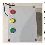
To manually interact with the entire system, a control box with three physical buttons was built.
