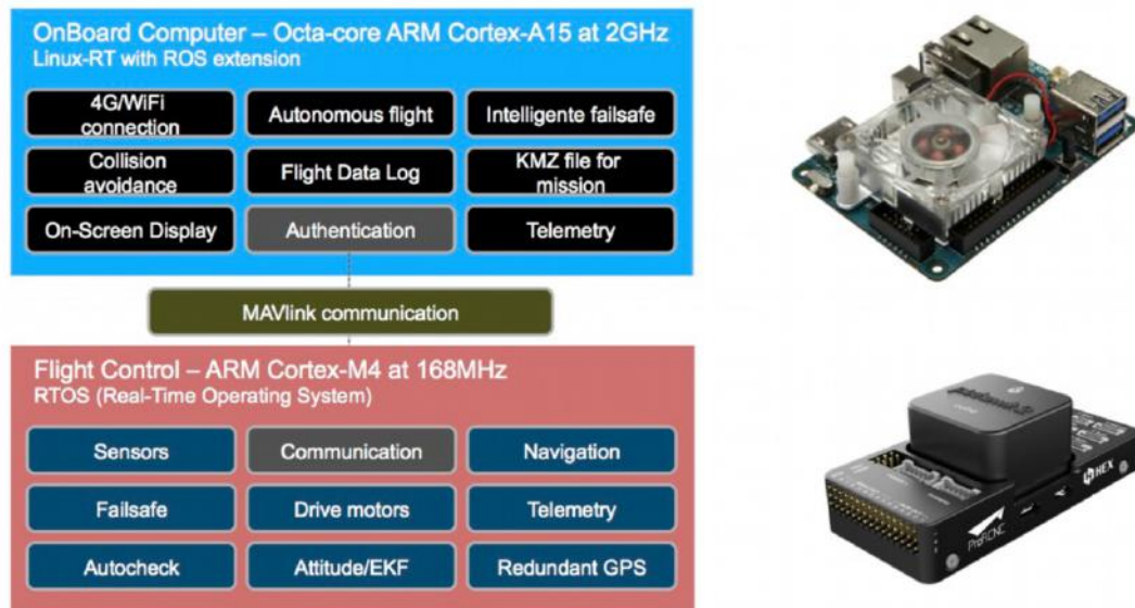
Figure 13: DigiSky's UAV architecture.
