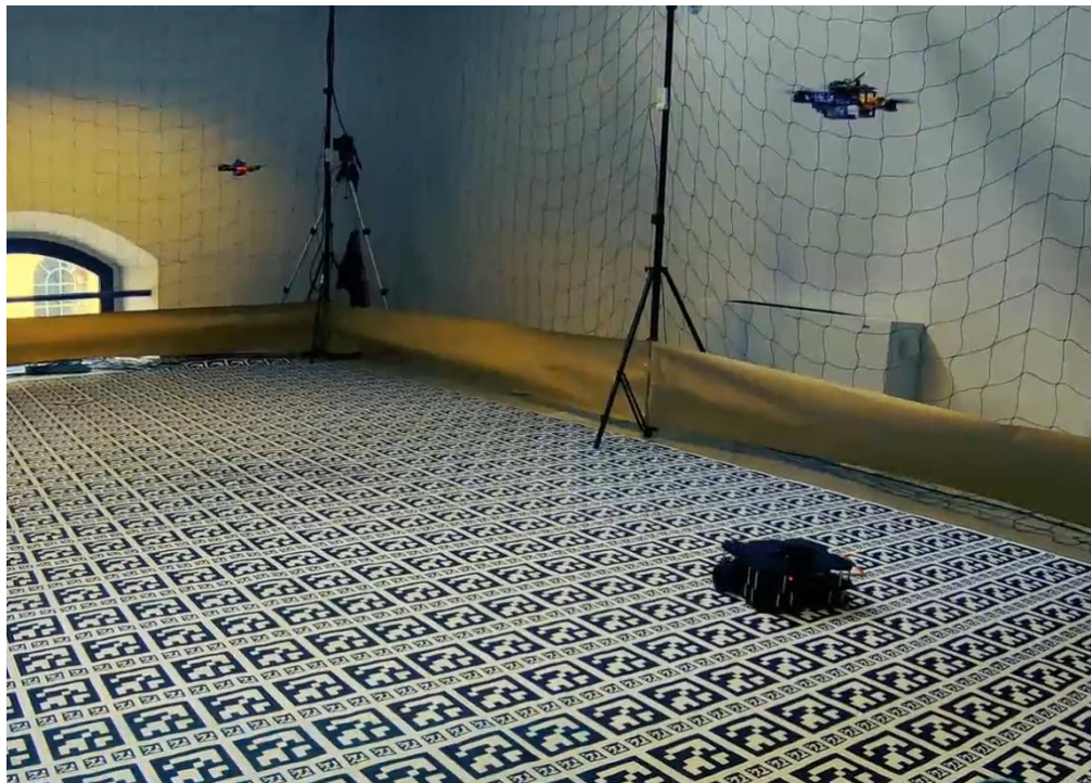
Figure 4 - Drone yaw estimation using AprilTags and video-camera
