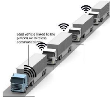
Figure 3: Vehicles in platooning configuration.
